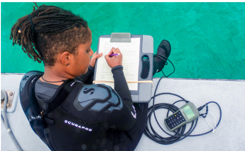
Using water quality samples data is being collected on its pH level, dissolved oxygen, temperature and light spectrum.
