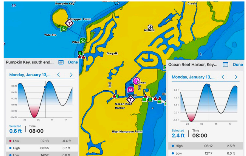
Tidal predictions displayed for Ocean Reef and Pumpkin Key for the morning of January 13, 2025. Tidal range and times in Card Sound are approximately 2 feet less than Ocean Reef and lag by nearly 3 hours. Charts illustrate negative low water predictions, known as "minus" tides.
